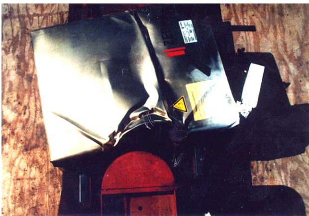
Fig. 7. ZEBRA battery type Z12–Crash Test at 50 km/h.
