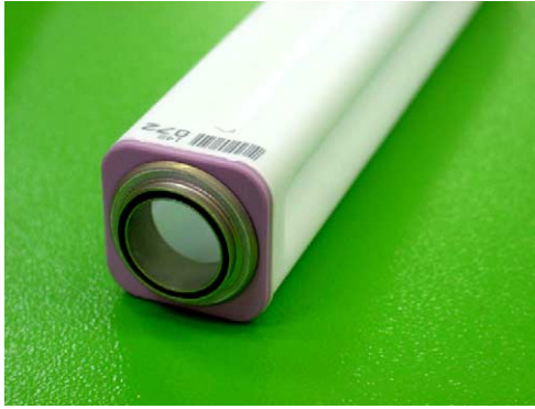
Fig. 3. \beta' ceramic with thermal compression bond (TCB) seal.
